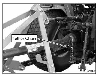
Figure 3. Attaching Mower to Tractor
